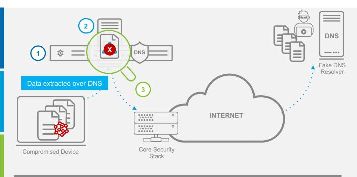
Attempted data exfiltration over DNS protocols detected and blocked
