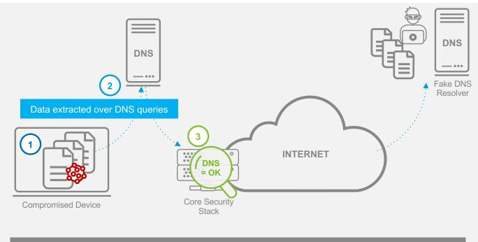
Sensitive data tunneled over DNS protocols avoid detection
