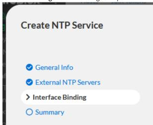
15. **Interface Bindings**: If desired you may select the interface the NTP service runs on. Note the NTP service can be bound to WAN, LAN, a custom interface label, or all interfaces. This setting is set to All Interface Binding by default.
