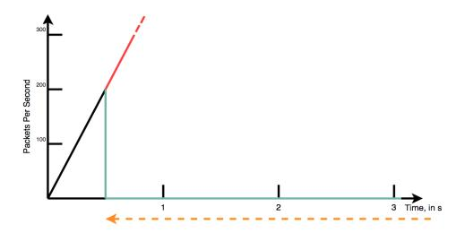
In the following diagram you see what occurs once we approach the end of the blocking period on second 2. The traffic rate during the last second, while still being blocked, is below 200 PPS. This means that as of second 2 traffic will be allowed again. If the traffic goes over 200 PPS again, the block would trigger and remain active until the client drops below the configured value.
